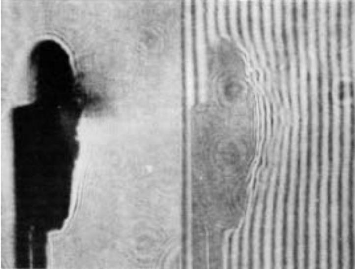
Fig. 43: Example of an interferogram and polarigram obtained simultaneously
